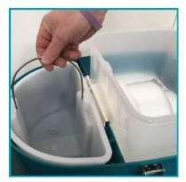
Empty and rinse both the solution and recovery tanks.
