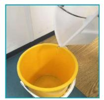
Make sure to empty the recovery tank when it is approximately  $\frac{3}{4}$  full. Do not refill the solution tank without emptying all the contents of the recovery tank first.
