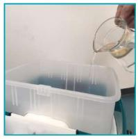
Add approx.  $\frac{1}{2}$  litre of clean water to solution tank to flush out the tank and pump.
